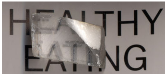
Fig. 3 A calcite crystal laid upon a paper with some letters showing the double refraction.
