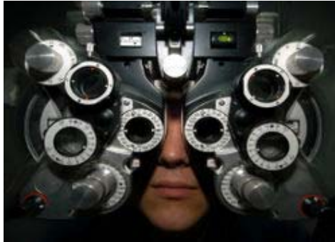
Fig. 1 An optical refractor, also called a phoropter in use.
