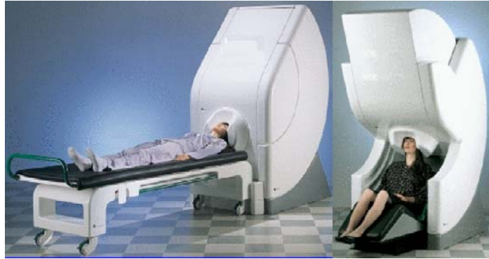
Fig. 1 MEG machine for operation in supine and sitting position of the subject
